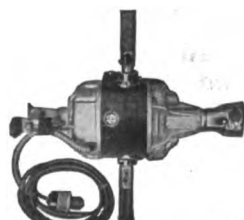
\frac{1}{2} " drill in steel, weight 24 pounds.
